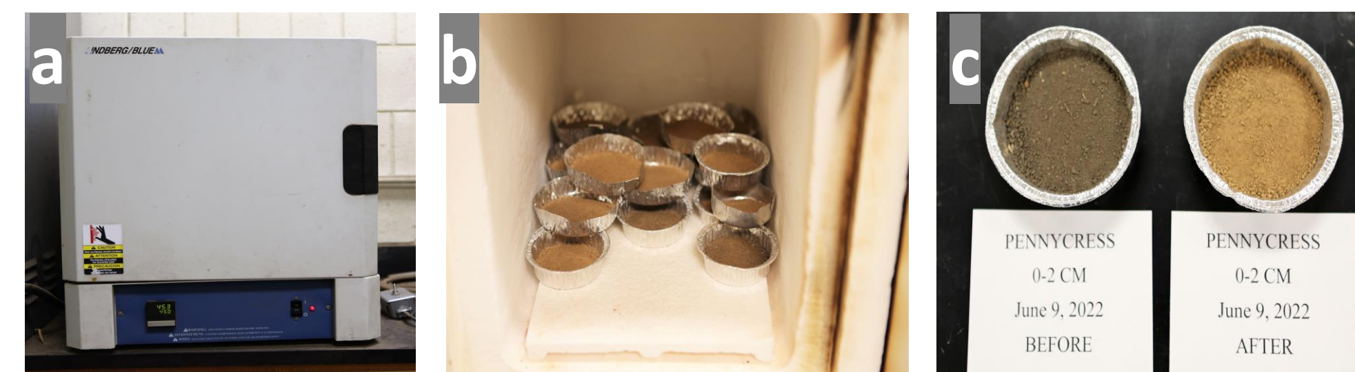
Figure 3: Soil organic matter was measured by loss on ignition after running soil samples in a muffle furnace (a & b) at 450 °C for 5 hours 9 (c).
